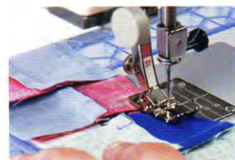
Feed pieces through the machine closely together and then cut the thread to separate them.
