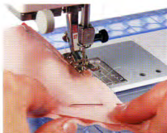
Sew from dot to dot, pivoting the fabric around the needle when you are ready to sew the next seam.
